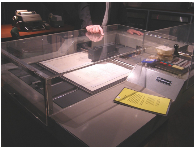
The Zuse Graphomat Z64, a plotter used by computer-art pioneers in the 1960s. Archive photograph, CC BY-SA.
