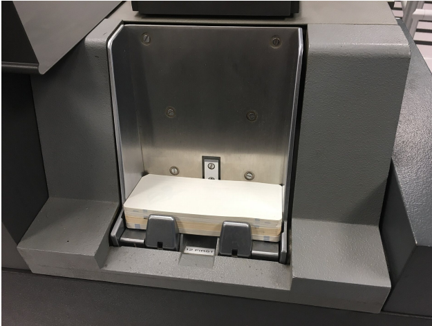
IBM 1402 card reader/punch: the material reality of mechanical classification. Photo Arnold Reinhold, CC BY-SA 3.0.
